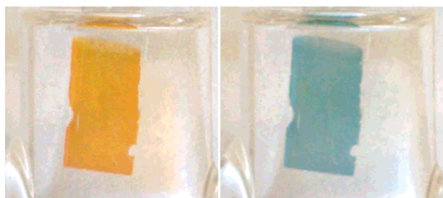
Figure 6. A three-layer film of electrochemically cross-linked 20-mer ROMP-poly1 changes from orange (left) to dark blue (right) in a perchlorate-containing electrolyte as the cell voltage is increased from -0.35 to 1.27 V. This dopant-induced color change is reversible over 20 or more cycles.
